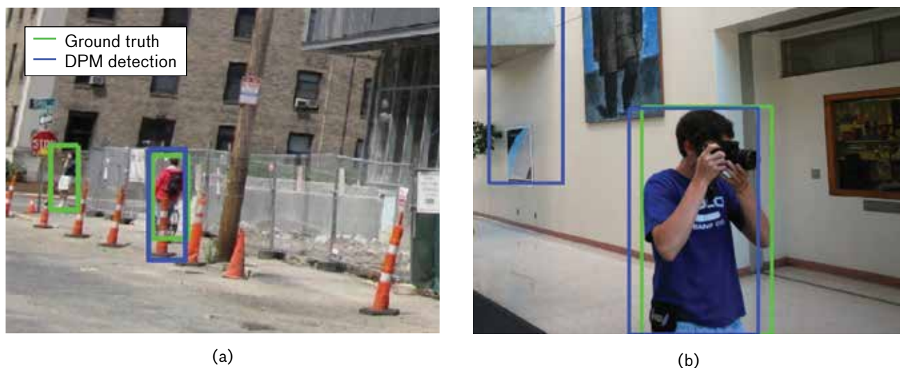
FIGURE 24. In (a), a traffic cone is incorrectly detected as part of a person, causing the DPM bounding box to be taller than the ground truth. This detection is still considered a true positive, but the 3D projection may be significantly shifted. In (b), DPM makes a partial detection that qualifies as a true positive.
