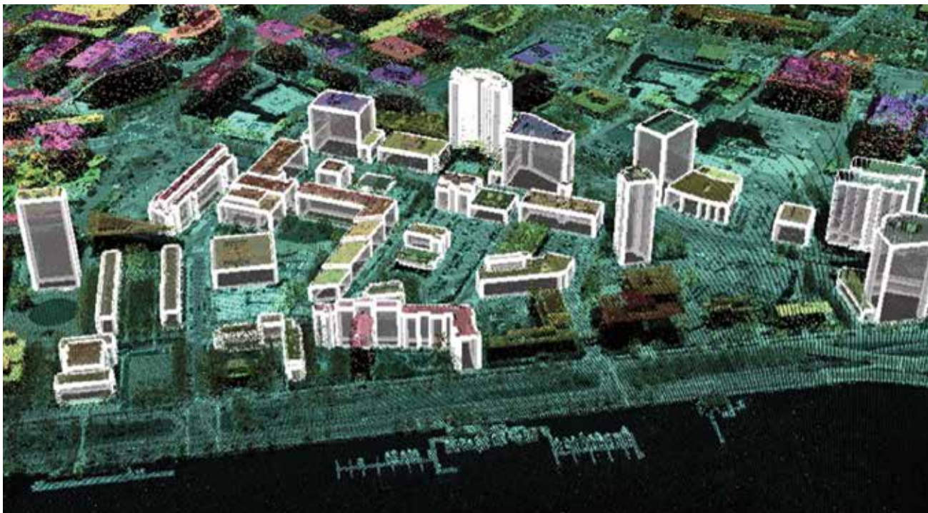
FIGURE 7. Building models are superposed against the lidar point cloud fused with the orthorectified aerial image.
