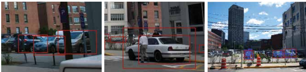
FIGURE 4. The DPM results show bounding boxes around cars occluded by other objects, e.g., person, pole, fence, or bushes.
