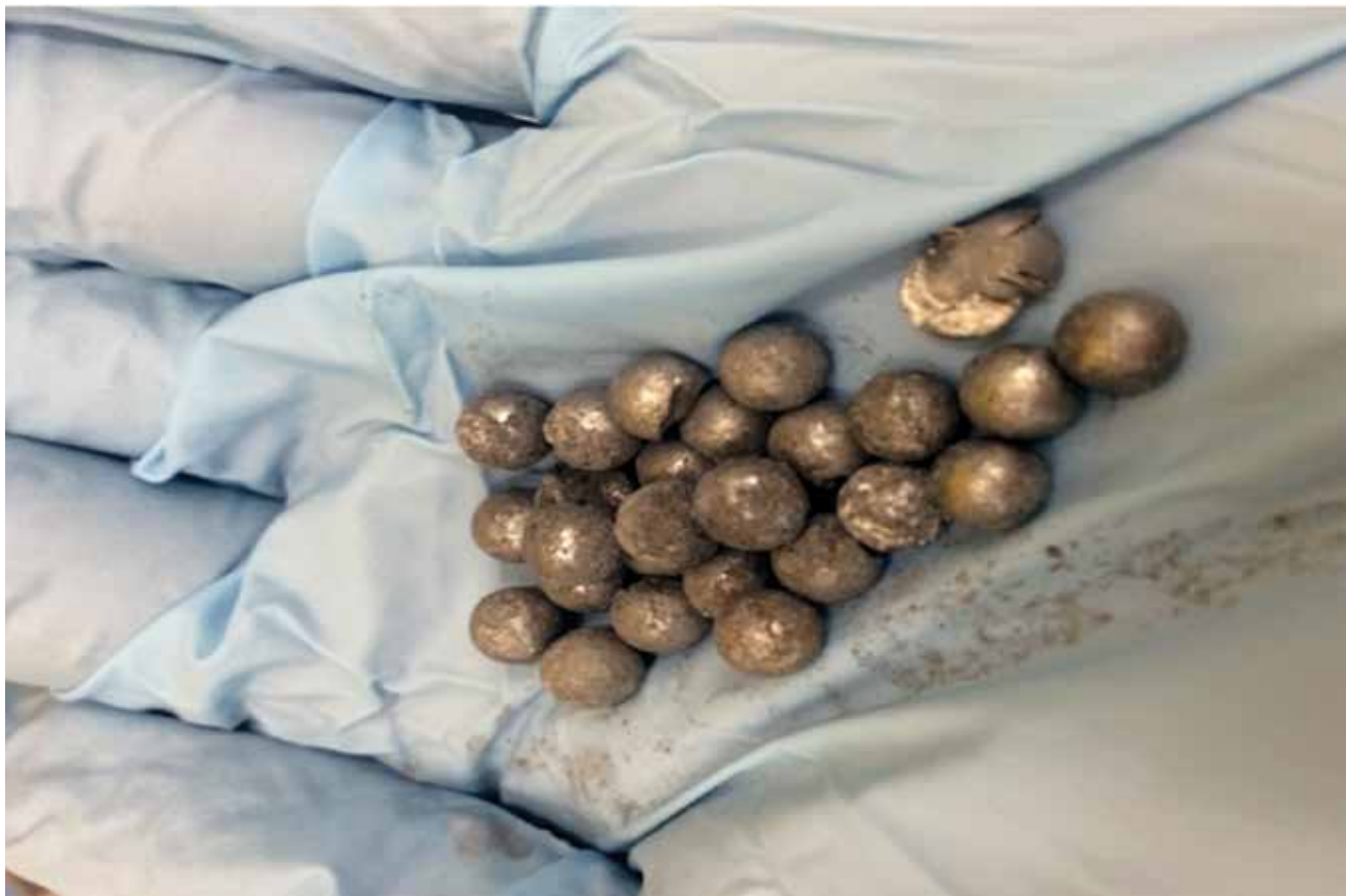
FIGURE 6. The dull surfaces of the 6 mm diameter aluminum pellets, shown after treatment with gallium, indium, and tin, are caused by the disruption of the aluminum oxide layer.
