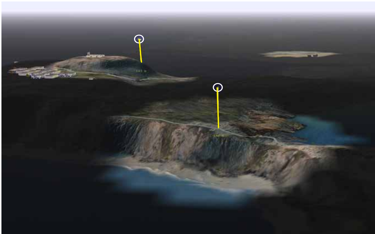
FIGURE 10. In this simulation, high-resolution sensors “paint” the terrain as the variances are reduced via data collection. The circles mark the locations of the UAVs and the yellow lines indicate the direction of the UAV sensors.
